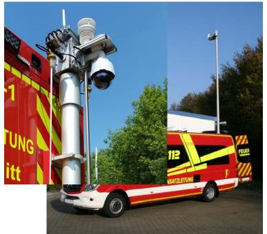
Mounted on a extendible mast at a fire engine in Germany.
